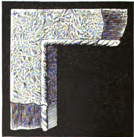
Fig. 193.—Section of Frame covered with Tin-foil
